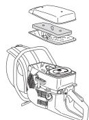
If the machine is low on power, difficult to start or runs poorly at idle speed: always check the spark plug first before taking any further action. If the spark plug is dirty, clean it and check that the electrode gap is 0.5 mm. The spark plug should be replaced after about a month in operation or earlier if necessary.
